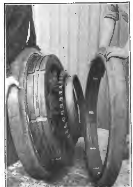
Fig. 3—Wheel with one tire in place and the other being put on
